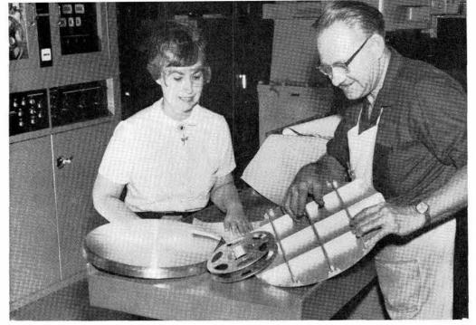
REBUILT MILLING MACHINE gives Livermore Model Shop capability of making three-dimensional parts by numeric control. Secretary Vivian Lenz observes while Model and Instruments Maker G. H. (Gus) Brockmoller (both 8223) shows the completed grid the machine made from a smooth aluminum disc. Converted mill and updated solid-state control panel can now fabricate parts  $10 \times 20 \times 30$  inches.
